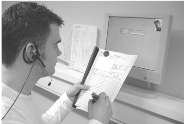
FIGURE 3. Users interact with NOSTOS by means of digital pens and special paper applications. Walk-up displays and mobile headsets provide feedback from the system.
